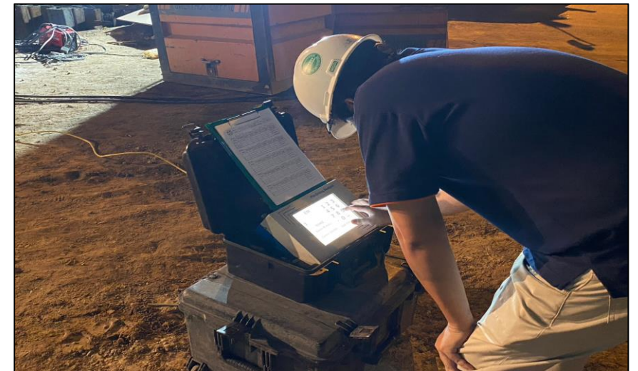
Dynamic Load test Barrette pile 3.00x1.00 m. MLP04-20L/1
